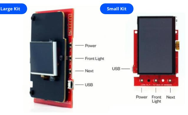
Displays used in development kits ARE NOT suitable for environmental testing.
