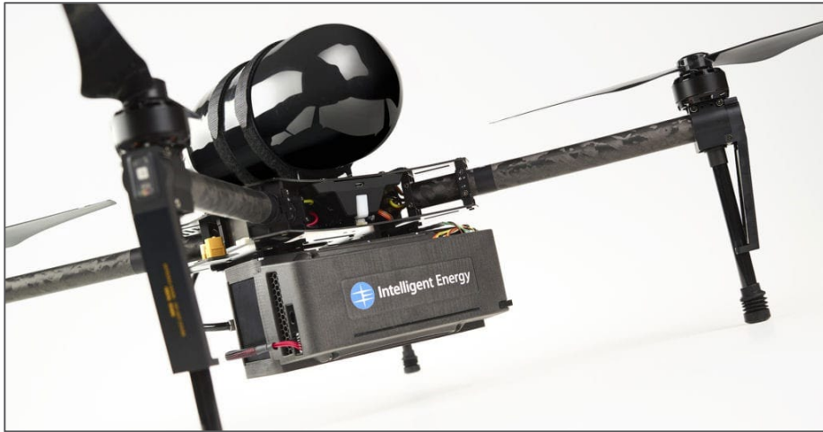
Hybrid Drones (Li-ion Batteries + Hydrogen FCs)
