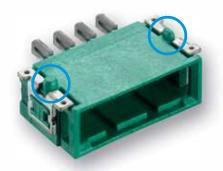
Two **pegs** (round and oval) ensures exact positioning on the PCB. In addition, they enable a compensation of the PCB hole tolerances.
