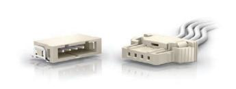
ERNI's iBridge Ultra is a 2mm pitch Single Row Connector that carries up to 8A per contact. Miniaturized, robust and powerful, connections are assured with dual locking sides and TPA.
