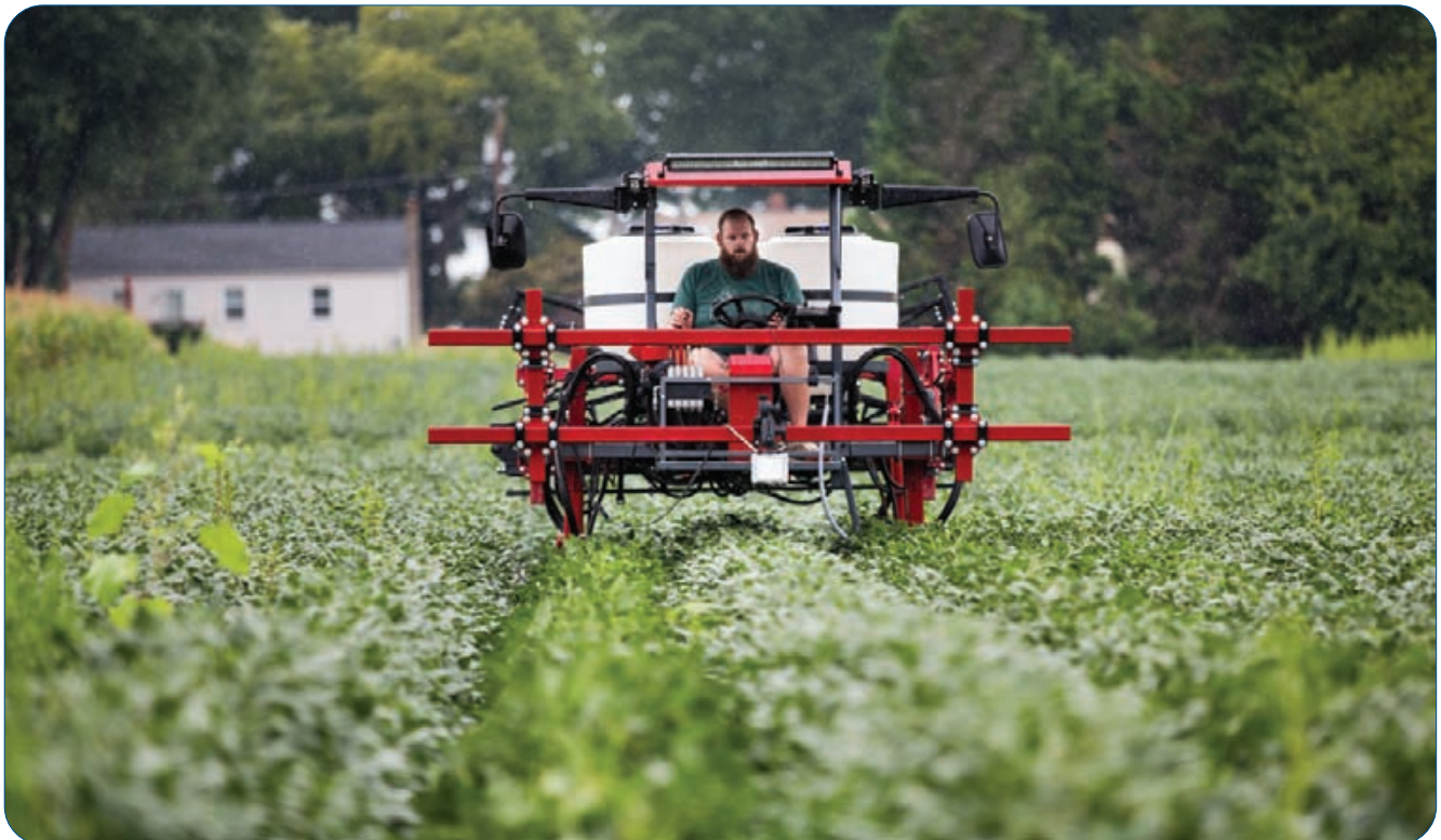
A highboy tractor equipped with sensors passes through a field at the USDA research farm in Beltsville. Photo courtesy of Microsoft
